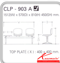
CLP - 903 A 1512W x 570D x 810H 450SH mm. TOP PLATE : 400 x 400 mm.
